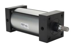
NITRA pneumatic cylinder, NFPA tie rod, 4in bore, 1in rod diameter, 6in stroke, double acting, magnetic piston, tapped end caps mount.
