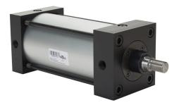
NITRA pneumatic cylinder, NFPA tie rod, 4in bore, 1in rod diameter, 6in stroke, double acting, magnetic piston, front and rear adjustable cushions, tapped end caps mount.
