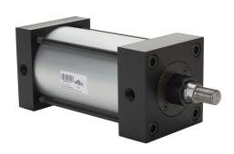
NITRA pneumatic cylinder, NFPA tie rod, 4in bore, 1in rod diameter, 5in stroke, double acting, magnetic piston, tapped end caps mount.
