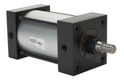
NITRA pneumatic cylinder, NFPA tie rod, 4in bore, 1in rod diameter, 4in stroke, double acting, magnetic piston, tapped end caps mount.
