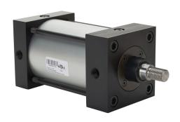
NITRA pneumatic cylinder, NFPA tie rod, 4in bore, 1in rod diameter, 4in stroke, double acting, magnetic piston, front and rear adjustable cushions, tapped end caps mount.
