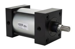
NITRA pneumatic cylinder, NFPA tie rod, 4in bore, 1in rod diameter, 3in stroke, double acting, magnetic piston, tapped end caps mount.
