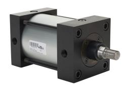
NITRA pneumatic cylinder, NFPA tie rod, 4in bore, 1in rod diameter, 3in stroke, double acting, magnetic piston, front and rear adjustable cushions, tapped end caps mount.
