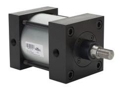
NITRA pneumatic cylinder, NFPA tie rod, 4in bore, 1in rod diameter, 2in stroke, double acting, magnetic piston, tapped end caps mount.
