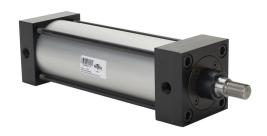
NITRA pneumatic cylinder, NFPA tie rod, 3-1/4in bore, 1in rod diameter, 8in stroke, double acting, magnetic piston, tapped end caps mount.
