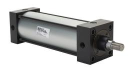
NITRA pneumatic cylinder, NFPA tie rod, 3-1/4in bore, 1in rod diameter, 8in stroke, double acting, magnetic piston, front and rear adjustable cushions, tapped end caps mount.
