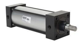
NITRA pneumatic cylinder, NFPA tie rod, 3-1/4in bore, 1in rod diameter, 7in stroke, double acting, magnetic piston, tapped end caps mount.
