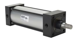
NITRA pneumatic cylinder, NFPA tie rod, 3-1/4in bore, 1in rod diameter, 7in stroke, double acting, magnetic piston, tapped end caps mount.
