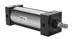
NITRA pneumatic cylinder, NFPA tie rod, 3-1/4in bore, 1in rod diameter, 7in stroke, double acting, magnetic piston, front and rear adjustable cushions, tapped end caps mount.
