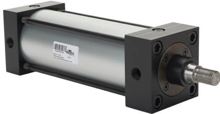
NITRA pneumatic cylinder, NFPA tie rod, 3-1/4in bore, 1in rod diameter, 7in stroke, double acting, magnetic piston, front and rear adjustable cushions, tapped end caps mount.
