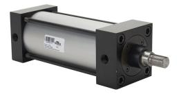
NITRA pneumatic cylinder, NFPA tie rod, 3-1/4in bore, 1in rod diameter, 6in stroke, double acting, magnetic piston, tapped end caps mount.
