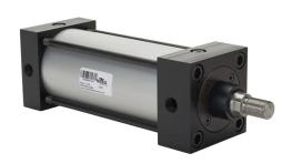
NITRA pneumatic cylinder, NFPA tie rod, 3-1/4in bore, 1in rod diameter, 6in stroke, double acting, magnetic piston, front and rear adjustable cushions, tapped end caps mount.
