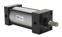
NITRA pneumatic cylinder, NFPA tie rod, 3-1/4in bore, 1in rod diameter, 5in stroke, double acting, magnetic piston, tapped end caps mount.
