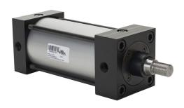
NITRA pneumatic cylinder, NFPA tie rod, 3-1/4in bore, 1in rod diameter, 5in stroke, double acting, magnetic piston, front and rear adjustable cushions, tapped end caps mount.
