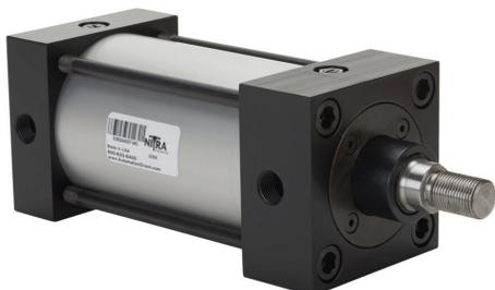
NITRA pneumatic cylinder, NFPA tie rod, 3-1/4in bore, 1in rod diameter, 4in stroke, double acting, magnetic piston, tapped end caps mount.
