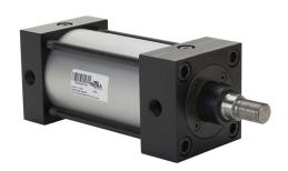
NITRA pneumatic cylinder, NFPA tie rod, 3-1/4in bore, 1in rod diameter, 4in stroke, double acting, magnetic piston, tapped end caps mount.
