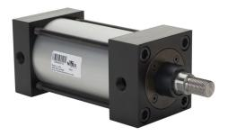
NITRA pneumatic cylinder, NFPA tie rod, 3-1/4in bore, 1in rod diameter, 4in stroke, double acting, magnetic piston, front and rear adjustable cushions, tapped end caps mount.
