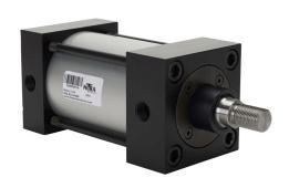
NITRA pneumatic cylinder, NFPA tie rod, 3-1/4in bore, 1in rod diameter, 3in stroke, double acting, magnetic piston, tapped end caps mount.
