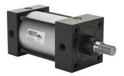
NITRA pneumatic cylinder, NFPA tie rod, 3-1/4in bore, 1in rod diameter, 3in stroke, double acting, magnetic piston, front and rear adjustable cushions, tapped end caps mount.
