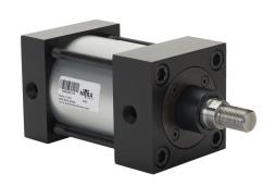
NITRA pneumatic cylinder, NFPA tie rod, 3-1/4in bore, 1in rod diameter, 2in stroke, double acting, magnetic piston, tapped end caps mount.
