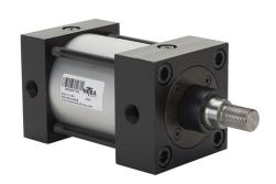
NITRA pneumatic cylinder, NFPA tie rod, 3-1/4in bore, 1in rod diameter, 2in stroke, double acting, magnetic piston, front and rear adjustable cushions, tapped end caps mount.
