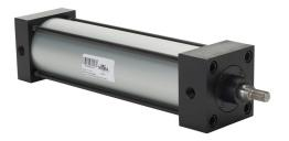
NITRA pneumatic cylinder, NFPA tie rod, 2-1/2in bore, 5/8in rod diameter, 8in stroke, double acting, magnetic piston, tapped end caps mount.
