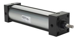
NITRA pneumatic cylinder, NFPA tie rod, 2-1/2in bore, 5/8in rod diameter, 8in stroke, double acting, magnetic piston, front and rear adjustable cushions, tapped end caps mount.
