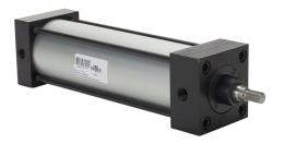
NITRA pneumatic cylinder, NFPA tie rod, 2-1/2in bore, 5/8in rod diameter, 7in stroke, double acting, magnetic piston, tapped end caps mount.
