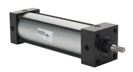
NITRA pneumatic cylinder, NFPA tie rod, 2-1/2in bore, 5/8in rod diameter, 7in stroke, double acting, magnetic piston, front and rear adjustable cushions, tapped end caps mount.
