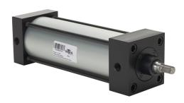
NITRA pneumatic cylinder, NFPA tie rod, 2-1/2in bore, 5/8in rod diameter, 6in stroke, double acting, magnetic piston, tapped end caps mount.
