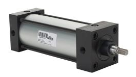
NITRA pneumatic cylinder, NFPA tie rod, 2-1/2in bore, 5/8in rod diameter, 5in stroke, double acting, magnetic piston, front and rear adjustable cushions, tapped end caps mount.
