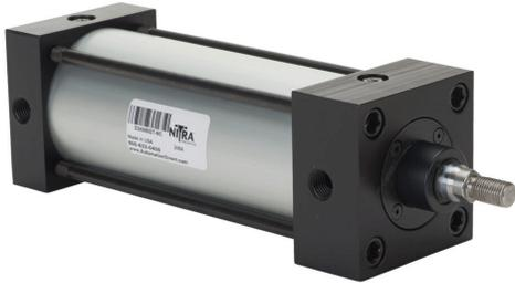
NITRA pneumatic cylinder, NFPA tie rod, 2-1/2in bore, 5/8in rod diameter, 5in stroke, double acting, magnetic piston, front and rear adjustable cushions, tapped end caps mount.
