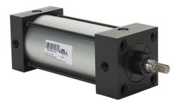
NITRA pneumatic cylinder, NFPA tie rod, 2-1/2in bore, 5/8in rod diameter, 4in stroke, double acting, magnetic piston, front and rear adjustable cushions, tapped end caps mount.
