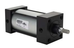
NITRA pneumatic cylinder, NFPA tie rod, 2-1/2in bore, 5/8in rod diameter, 3in stroke, double acting, magnetic piston, tapped end caps mount.
