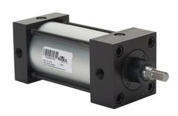
NITRA pneumatic cylinder, NFPA tie rod, 2-1/2in bore, 5/8in rod diameter, 3in stroke, double acting, magnetic piston, front and rear adjustable cushions, tapped end caps mount.
