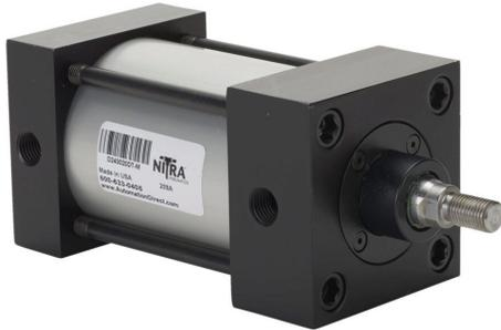
NITRA pneumatic cylinder, NFPA tie rod, 2-1/2in bore, 5/8in rod diameter, 2in stroke, double acting, magnetic piston, tapped end caps mount.
