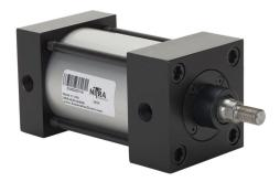
NITRA pneumatic cylinder, NFPA tie rod, 2-1/2in bore, 5/8in rod diameter, 2in stroke, double acting, magnetic piston, tapped end caps mount.
