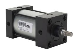
NITRA pneumatic cylinder, NFPA tie rod, 2-1/2in bore, 5/8in rod diameter, 2in stroke, double acting, magnetic piston, front and rear adjustable cushions, tapped end caps mount.
