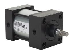
NITRA pneumatic cylinder, NFPA tie rod, 2-1/2in bore, 5/8in rod diameter, 1in stroke, double acting, magnetic piston, tapped end caps mount.
