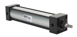
NITRA pneumatic cylinder, NFPA tie rod, 2in bore, 5/8in rod diameter, 8in stroke, double acting, magnetic piston, tapped end caps mount.
