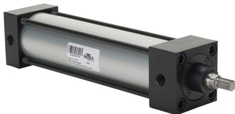
NITRA pneumatic cylinder, NFPA tie rod, 2in bore, 5/8in rod diameter, 7in stroke, double acting, magnetic piston, tapped end caps mount.
