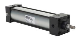
NITRA pneumatic cylinder, NFPA tie rod, 2in bore, 5/8in rod diameter, 7in stroke, double acting, magnetic piston, front and rear adjustable cushions, tapped end caps mount.
