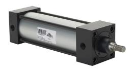
NITRA pneumatic cylinder, NFPA tie rod, 2in bore, 5/8in rod diameter, 5in stroke, double acting, magnetic piston, tapped end caps mount.
