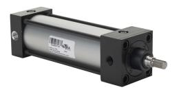
NITRA pneumatic cylinder, NFPA tie rod, 2in bore, 5/8in rod diameter, 5in stroke, double acting, magnetic piston, front and rear adjustable cushions, tapped end caps mount.
