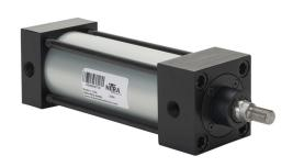
NITRA pneumatic cylinder, NFPA tie rod, 2in bore, 5/8in rod diameter, 4in stroke, double acting, magnetic piston, tapped end caps mount.
