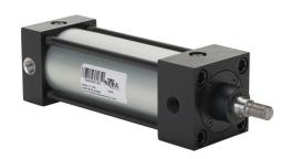
NITRA pneumatic cylinder, NFPA tie rod, 2in bore, 5/8in rod diameter, 4in stroke, double acting, magnetic piston, front and rear adjustable cushions, tapped end caps mount.
