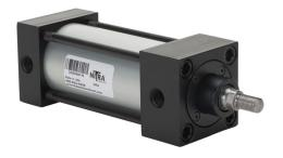
NITRA pneumatic cylinder, NFPA tie rod, 2in bore, 5/8in rod diameter, 3in stroke, double acting, magnetic piston, tapped end caps mount.
