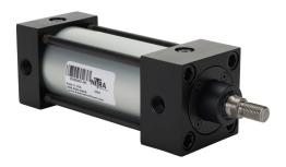
NITRA pneumatic cylinder, NFPA tie rod, 2in bore, 5/8in rod diameter, 3in stroke, double acting, magnetic piston, front and rear adjustable cushions, tapped end caps mount.
