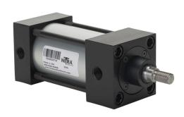
NITRA pneumatic cylinder, NFPA tie rod, 2in bore, 5/8in rod diameter, 2in stroke, double acting, magnetic piston, tapped end caps mount.
