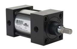
NITRA pneumatic cylinder, NFPA tie rod, 2in bore, 5/8in rod diameter, 1in stroke, double acting, magnetic piston, tapped end caps mount.
