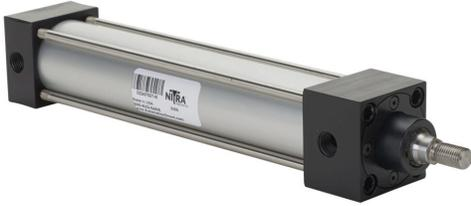
NITRA pneumatic cylinder, NFPA tie rod, 1-1/2in bore, 5/8in rod diameter, 7in stroke, double acting, magnetic piston, tapped end caps mount.
