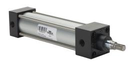
NITRA pneumatic cylinder, NFPA tie rod, 1-1/2in bore, 5/8in rod diameter, 5in stroke, double acting, magnetic piston, tapped end caps mount.
