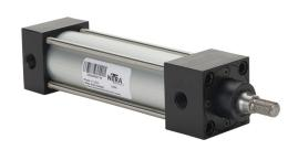
NITRA pneumatic cylinder, NFPA tie rod, 1-1/2in bore, 5/8in rod diameter, 4in stroke, double acting, magnetic piston, tapped end caps mount.
