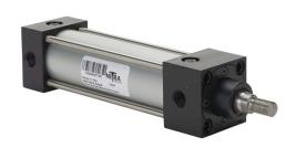
NITRA pneumatic cylinder, NFPA tie rod, 1-1/2in bore, 5/8in rod diameter, 4in stroke, double acting, magnetic piston, front and rear adjustable cushions, tapped end caps mount.
