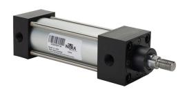
NITRA pneumatic cylinder, NFPA tie rod, 1-1/2in bore, 5/8in rod diameter, 3in stroke, double acting, magnetic piston, tapped end caps mount.
